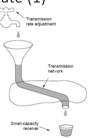
A fast network feeding a low-capacity receiver → flow control is needed
