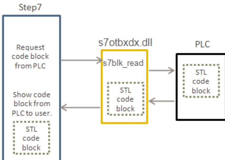
As mentioned previously, the Step 7 software uses a library file called s7otbxdx.dll to perform the actual communication with the PLC. The Step7 program calls different routines in this .dll file when it wants to access the PLC. For example, if a block of code is to be read from the PLC using Step7, the routine s7blk\_read is called. The code in s7otbxdx.dll accesses the PLC, reads the code, and passes it back to the Step7 program, as shown in figure 22.
