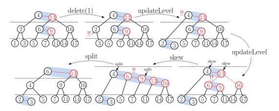
Fig. 7: Example of AA-tree deletion. (Remember, a node is red if it is at the same level as its parent.)
