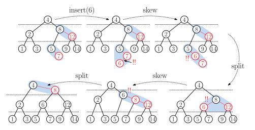
Fig. 6: Example of AA-tree insertion. (Remember, a node is red if it is at the same level as its parent.)
