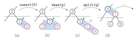
Fig. 5: AA insertion: (a) Initial tree, (b) after insertion, (c) after skewing, (d) after splitting.
