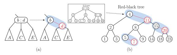
Fig. 1: Encoding a 2-3 tree as an equivalent binary tree.
