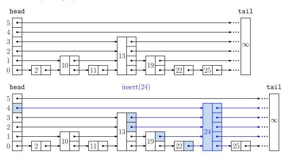
Fig. 5: Inserting a new key 24.
