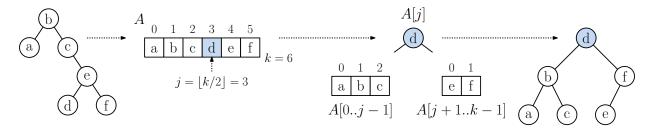
Fig. 1: Recursively building a balanced tree from a sorted array of keys.
