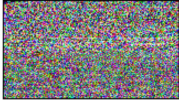
**Fig. 3.** A modulated CovertCast image for use in YouTube. Every colored block is  $8 \times 8$  pixels and encodes 6 bits of data.
