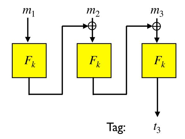
Secure only if length fixed. Otherwise, Eve can get the tags  $t_1$ ,  $t_2$ , etc. by querying the oracle for messages  $m_1$ , then  $m_1 || m_2$ , etc.
