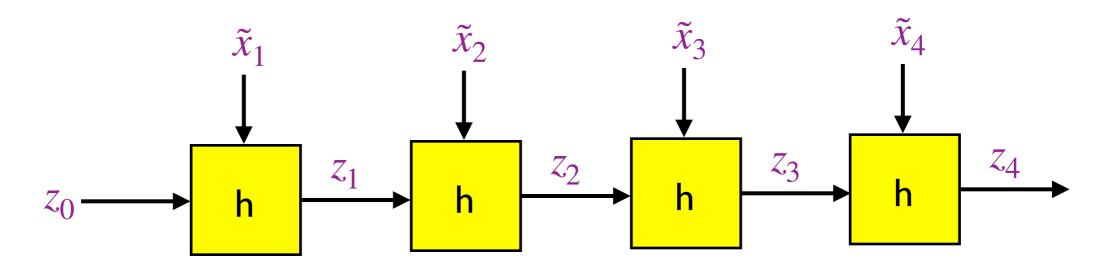
Theorem: If h(z,x) is collision-resistant, then H(x) given by the Merkle-Damgard construction is collision-resistant as well.
