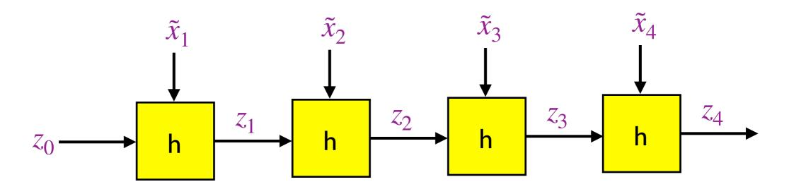
Theorem: If h(z,x) is collision-resistant, then H(x) given by the Merkle-Damgard construction is collision-resistant as well.
