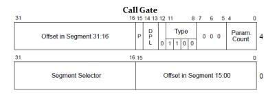
• While transferring control to the proper segment, the processor clears the EFLAGS.IF flag, thus disabling further maskableinterrupts.
