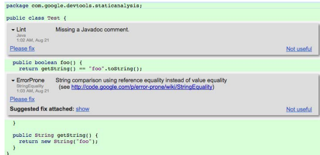
Fig. 3: Screenshot of analysis results; changelist reviewer view. In this case there are two results: one from the Java Lint tool (configured version of checkstyle [9]), and one from ErrorProne [17]. Reviewers can click on the NOT USEFUL link if they have a problem with the analysis results. They can also click on PLEASE FIX to indicate that the author should fix the result. They can also view the attached fix (Figure 4).
