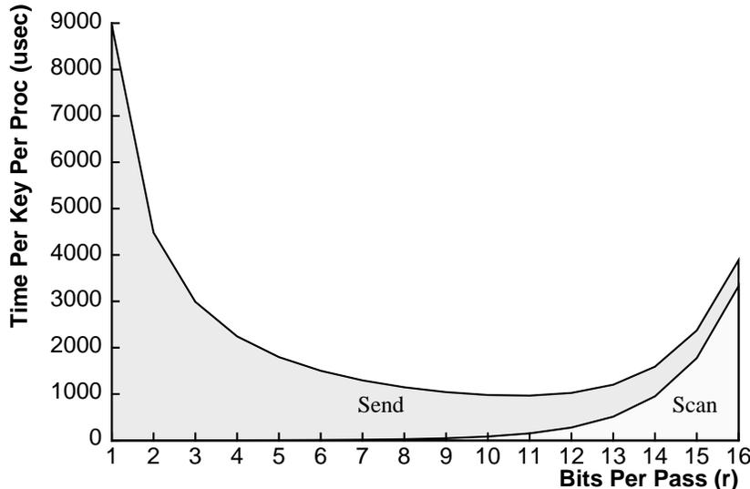
**Figure 7:** A breakdown of the total running time of radix sort into send time and scan time for sorting 64-bit keys ( $b = 64$ ) with  $n/p = 4096$ . The total running time is indicated by the top curve. The two shaded areas represent the scan time and send time. As  $r$  is increased, the scan time increases and the send time decreases. (The arithmetic time is negligible.) For the parameters chosen, the optimal value of  $r$  is 11.
