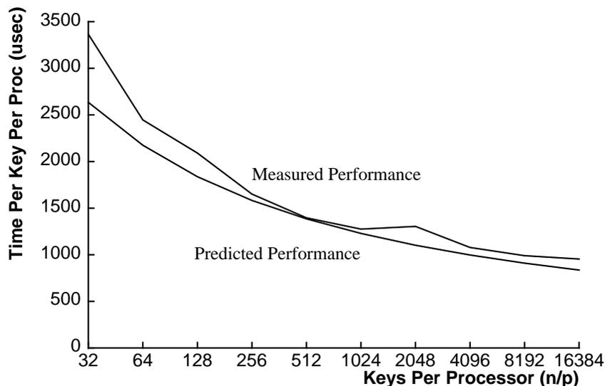
**Figure 8:** Predicted and measured performance of radix sort with 64-bit keys. Measured performance is on a 32K CM-2 and uses the empirically determined optimal values for  $r$ . Predicted performance was calculated using equation (8).
