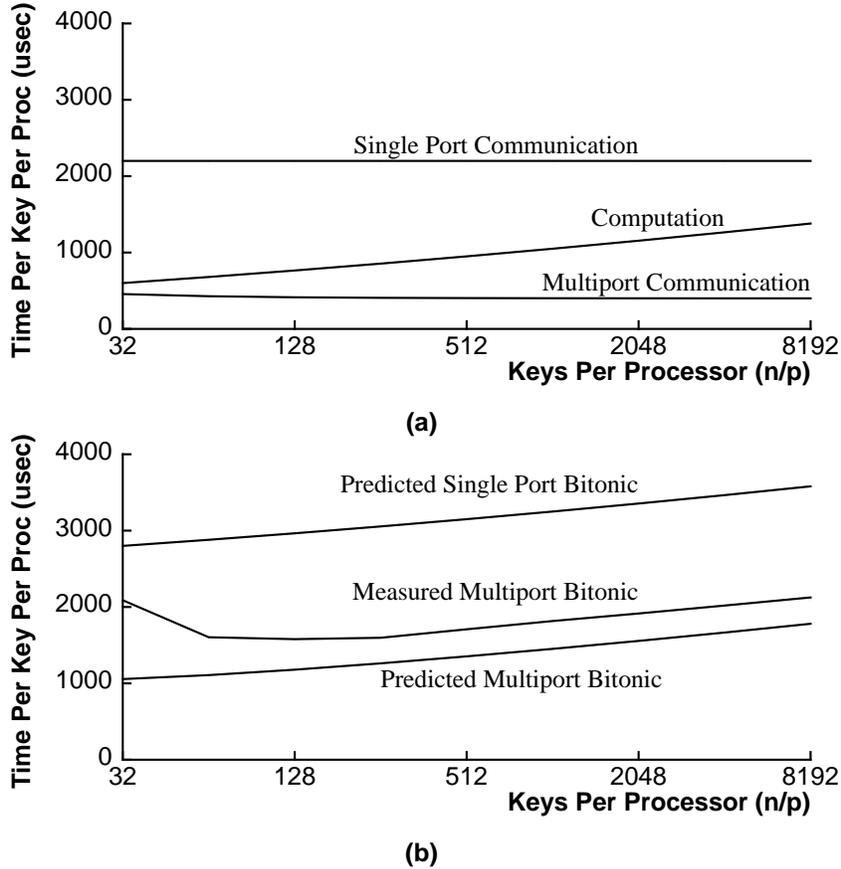
**Figure 6:** Bitonic sorting 64-bit keys on a 32K CM-2 ( $p = 1024$ ). (a) The predicted single port communication is approximately 5 times the predicted multiport communication time. (b) The measured performance of multiport bitonic sort closely matches the predicted performance, but contains a fixed overhead.
