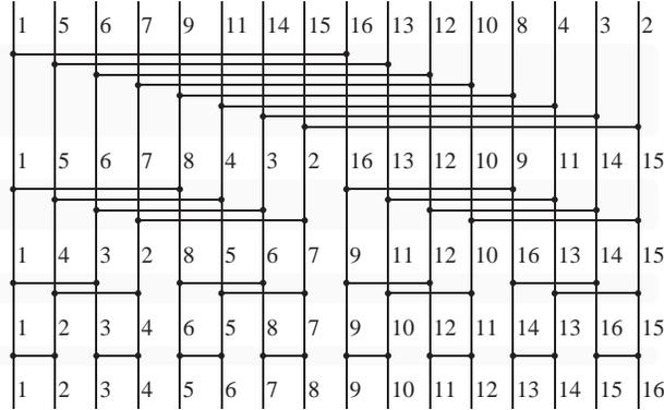
**Figure 5:** Viewing the BITONIC-MERGE procedure as a hypercube algorithm. Each vertical line represents a hypercube processor. Each horizontal line segment represents the communication of keys along the hypercube wire between two processors.
