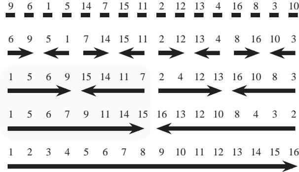
**Figure 4:** An illustration of the BITONIC-SORT procedure. Each arrow represents a sequence of keys sorted in the direction of the arrow. The unsorted input sequence of  $n$  keys is shown at the top, and the sorted output sequence is shown at the bottom. A bitonic merge operation is shaded. During the  $d$ th step of the algorithm,  $n/2^{d+1}$  merges are performed, each producing a bitonic sequence of length  $2^{d+1}$  from two bitonic sequences of length  $2^d$ .
