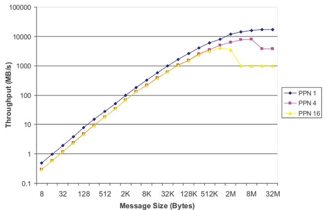
Figure 10. Broadcast throughput on 2048 nodes via the multi-color rectangle broadcast algorithm
