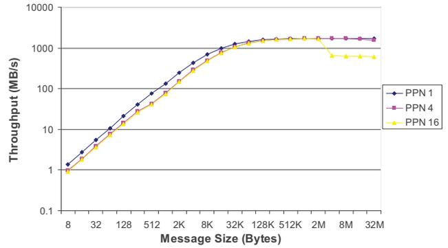
Figure 9. Broadcast throughput via collective network on 2048 nodes
