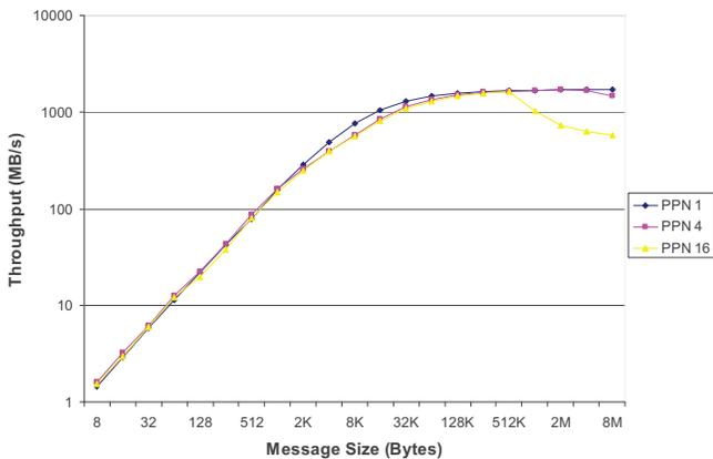
Figure 8. Allreduce throughput via collective network on 2048 nodes (MPI\_DOUBLE, MPI\_SUM)
