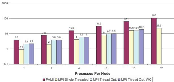
Figure 5. PAMI and MPI message rate (MMPS) on 32 nodes.
