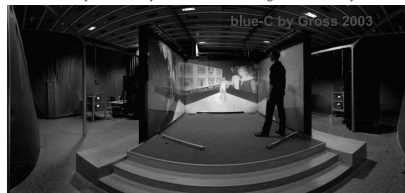
Figure 3: Picture illustrating the projector-camera arrangement of blue-c. a) Schematic view. b) Real system with scaffold to attach the cameras.
