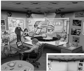
Figure 1: A conceptual sketch of the office of the future. By replacing the normal office lights with projectors, one could obtain precise control over all of the light in the office. With the help of synchronized cameras, the geometry and reflectance information can be captured for all of the visible surfaces in the office so that one can project images on the surfaces, render images of the surfaces, or interpret changes in the surfaces. The inset image is intended to help differentiate between the projected images and the real objects in the sketch.
