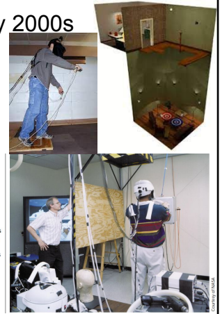
3 NASA-Houston's "Charlotte" Virtual Weightless Mass lets astronauts practice handling weightless massy objects.
