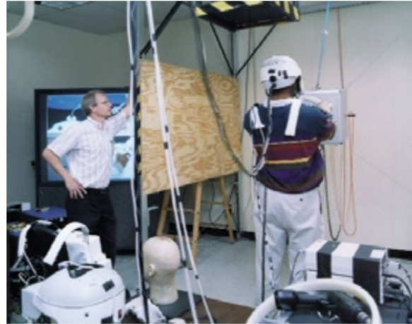
3 NASA-Houston's "Charlotte" Virtual Weightless Mass lets astronauts practice handling weightless massy objects.
