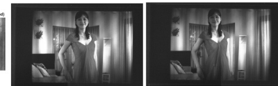
Figure 8: Pictures of images displayed by the experimental system taken at corresponding position of exit pupil; (a) image for left eye and (b) for right eye.
