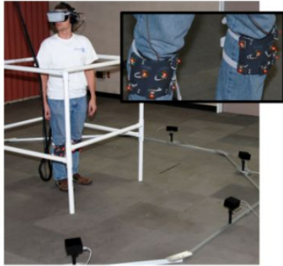
Figure 11: A user within the UNC GUD WIP system. The user wears beacons for 6-DOF trackers on his shins (inset). Shin-tracking cameras surround the subject on the floor. The user's heel position is approximated by rigid-body transform from the shin's pose.
