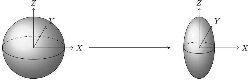
Figure 1.2: Bloch sphere transformation induced by a dephasing channel
