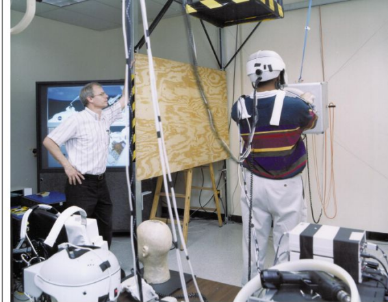
3 NASA-Houston's "Charlotte" Virtual Weightless Mass lets astronauts practice handling weightless massy objects.
