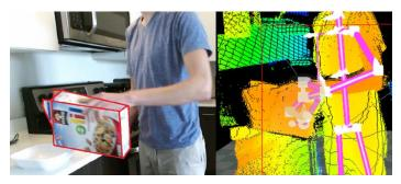
*Figure B:* Left shows a much clearer RGB image that provides much better views for texture-based recognition. Right shows depth point cloud which is much more accurate from this view.
