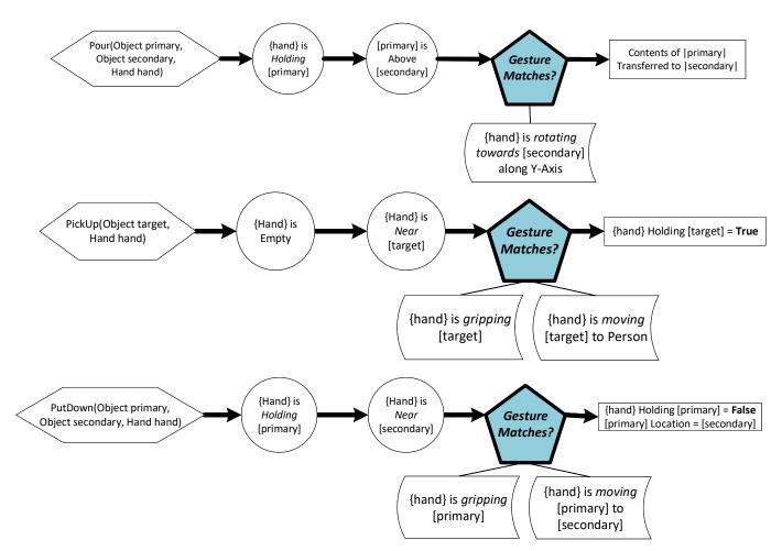
**Figure D:** Actions B and C being performed with Object and Gesture Recognition, to find the Action that best matches based on domain knowledge and the current state of the environment.
