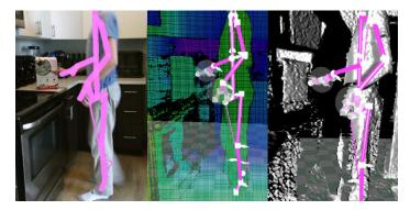
*Figure A:* In the above image, a human is reaching for a cereal box, but due to the camera angle and distance, it is difficult for the system to make an accurate prediction about the cereal box, until it is brought into a better view as shown in *Figure B*.
