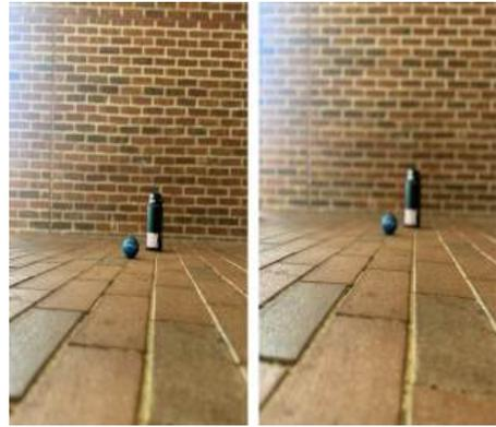
**Figure 4:** The static scene experimental setup with defocus blur at different depths in the scene. Left: the ball, water bottle, and brick wall are in focus while the floor is defocused. Right: parts of the floor is in focus while the ball, water bottle and brick wall are defocused.
