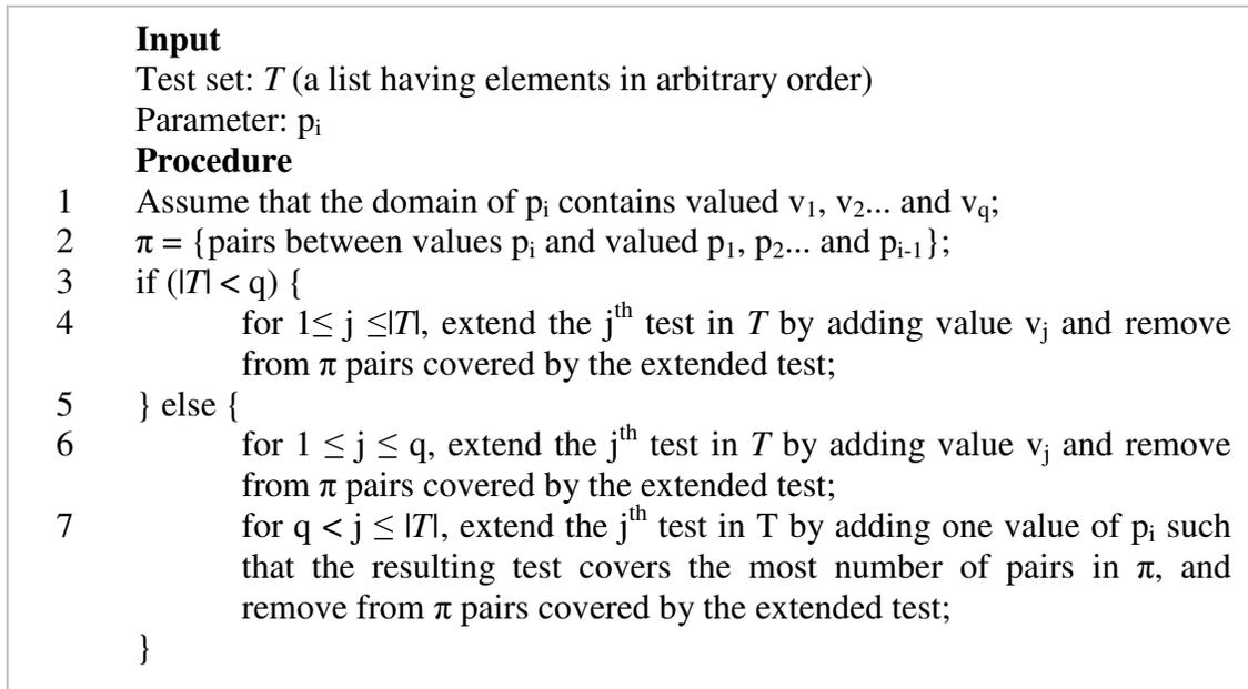
Figure 3: Algorithm  $IPO\_H(T, P_i)$  for horizontal growth
