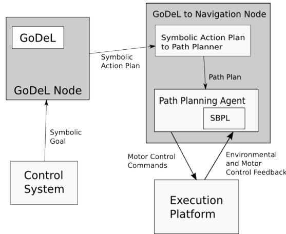
Figure 2: System Architecture: Integrating GoDeL with the SBPL
