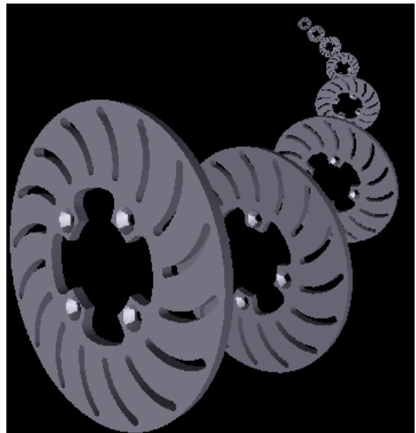
Figure 1: A level-of-detail hierarchy for the rotor from a brake assembly.
