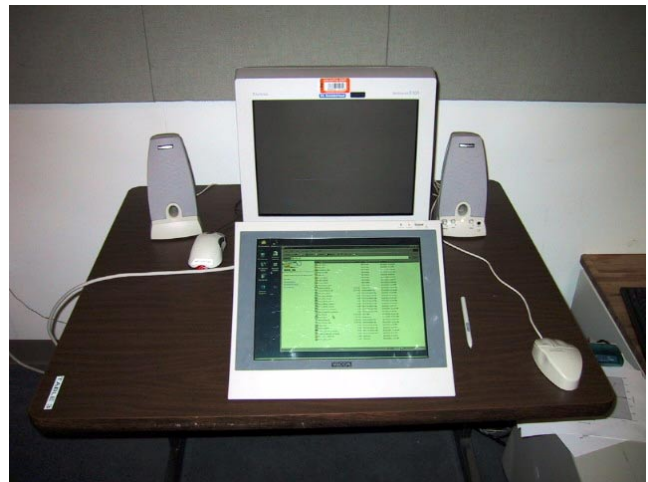
Figure 5: Experimental setting showing the mouse (front right), the Wacom PL400 (front) used as a tablet in direct and indirect conditions, and the display (rear) used for indirect conditions.
