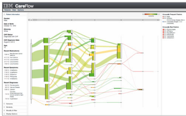
Fig. 2. Rather than visualizing all patients, CareFlow [46] employs a Goal-Driven Record Extraction strategy (S1) to focus users on only the most relevant 300 patients by applying similarity analytics, which results in a comprehensible flow graph of only 47 nodes and 111 edges.
