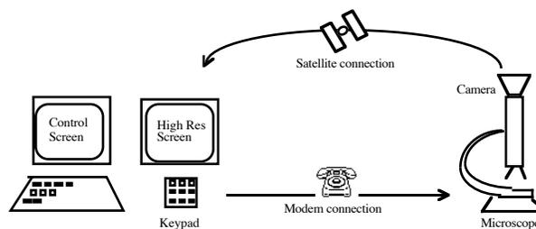
Figure 1 -- Simplified diagram of an existing telepathology system.
