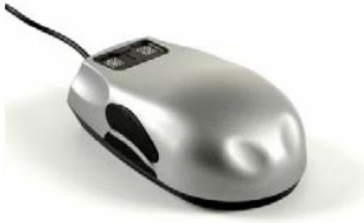
Figure 2-2 : The VTPlayer tactile mouse is equipped with two 4x4 mechanical matrix units that can be used to deliver a tactile sense of the screen. For example, as users explore a U.S. map, the tactile patterns change over different states.
