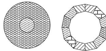
Figure 2: Relative brightness and spiculation detection filters: the left filter calculates the percent of the pixels in the outer ring that are less bright than the least bright of the pixels in the inner disk. The filter highlights the areas of the image that have bright cores, a characteristic of spiculated lesions. Multiple sizes are used because the sizes of the cancers vary. The right filter is used to detect spiculation, or radiating lines out of the core.
