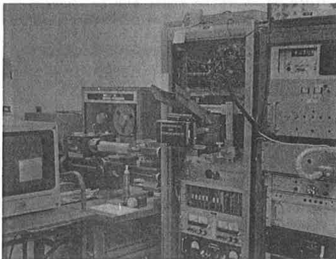
Digitizing and display equipment. The scanner is the horizontal drum in front of the tape drive. Storage and display circuits are housed in the racks, and the camera is on the left rack. Pictures can also be displayed on the TV monitor at the left.
