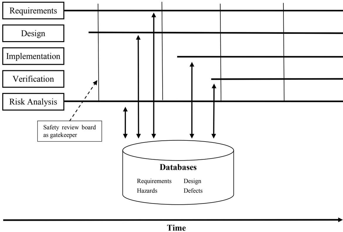
Figure 2. NASA safety monitoring process
