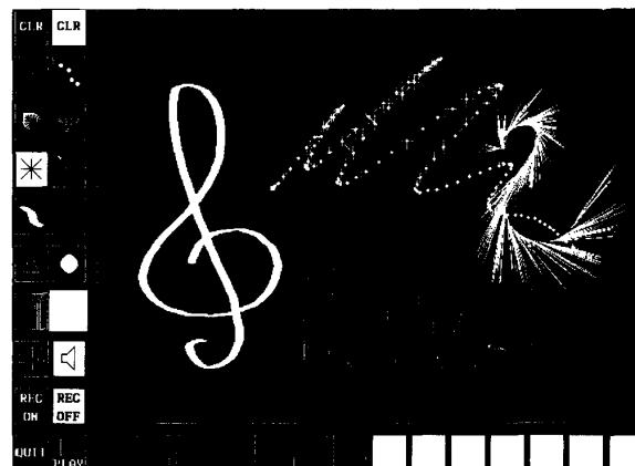
Figure 4. The Playpen tool combines traditional touch-and-select technology with velocity and motion sensing. This added information can be used to control volume, pitch, brightness, speed and other such attributes.
