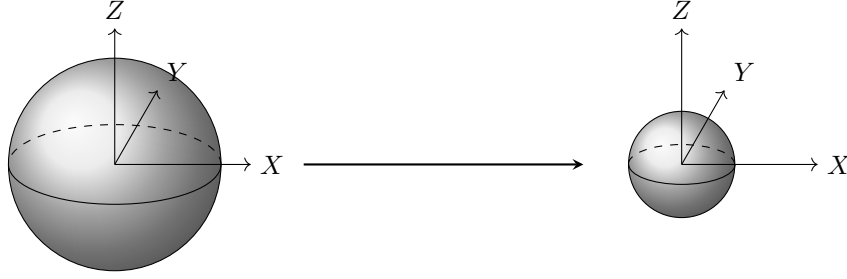
Figure 1.4: Bloch sphere transformation induced by a depolarizing channel
