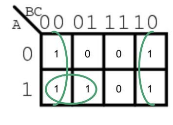
Output:  $A\overline{B} + \overline{C}$
