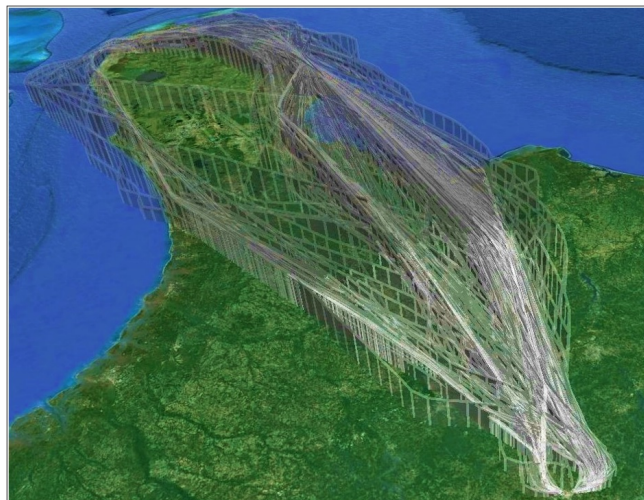
Figure 2: 3D raw trajectories of flight DAL2173 for the period of May 2010 through December 2015 in Google Earth. Climb phase is colored white, cruise and descent phases are colored gray.
