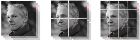
Figure 1: Illustration of the pyramid structure and color channel segments which are used to compute the hierarchical color histograms.
