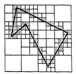
Fig. 5. MX quadtree corresponding to Figure 4.
