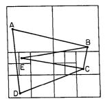
Fig. 8. PM<sub>2</sub> quadtree meeting criteria C1, C2', and C3'.
