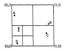
Fig. 3. PR quadtree corresponding to the vertices A, B, C, D, and E, of polygonal map of Figure 2.
