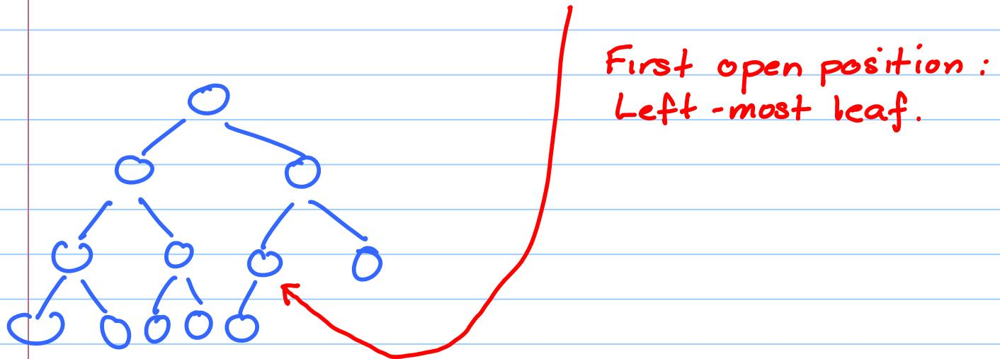
The challenge is to maintain [in  $O(\log n)$  time] the heap's overall property of subtrees having contents less than (or for a Min Heap greater than) the local root node.
