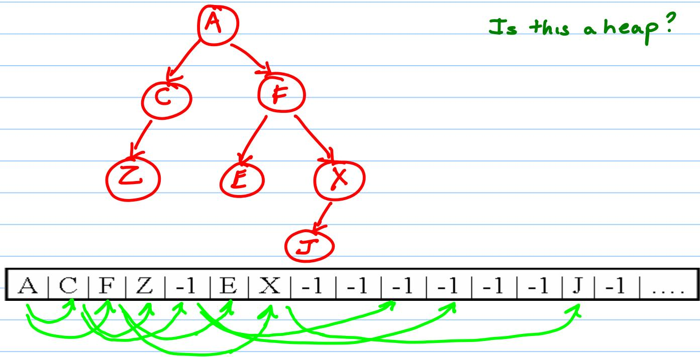
When used with complete trees such as heaps, there are no gaps within the tree — only empty spaces on the extreme right.
