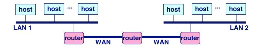
LAN 1 and LAN 2 might be completely different, totally incompatible LANs (e.g., Ethernet and ATM)
