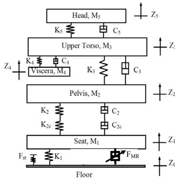
**Figure 1 – Mechanical Model of Seat Suspension System Coupled with a Human Body in Seated Posture**
