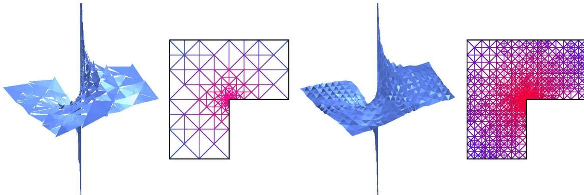
Stokes flow over an L-shaped domain: Pressures and meshes for error tolerance of 5% and unstable finite element pairs (resp. DOFs):  $\mathcal{P}^2\text{-}\mathcal{P}_d^1$  (1940),  $\mathcal{P}^1\text{-}\mathcal{P}^1$  (4971). The oscillations do not persist under further selective refinement (nonlinear stabilization effect of adaptivity). Error estimation and adaptivity will be fully discussed in this course.
