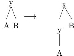
3. *Delete*( $x$ ) - Run *splay*( $x$ ) on the tree to bring  $x$  to the top. Then run *splay*( $x$ ) again in  $x$ 's left subtree  $A$  to bring  $y$ , the largest element less than  $x$ , to the top of  $A$ .  $y$  will have an empty right subtree in  $A$  since it is the largest element there. Then it is trivial to join the pieces together again without  $x$ :
