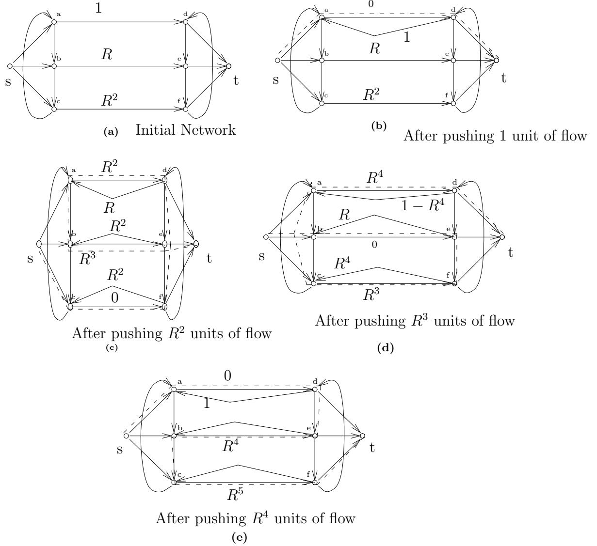
Figure 17: Non-terminating Example
