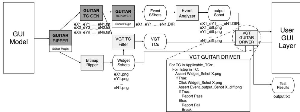
Fig. 1: Visualization of VGT GUITAR’s architecture. Squares show code components of the tool and rounded squares show artifacts generated by said components.
