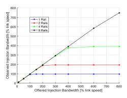
Fig. 2: Multi-rail verification using a synthetic bisectionpairing workload. The axes show the offered and observed injection bandwidth in percent of the link speed of EDR InfiniBand (12.5 GB/s).
