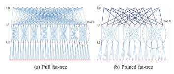
Fig. 1: Example configurations of (a) full and (b) pruned 3-level fat-trees using 8-port switches yielding 128 and 48 compute nodes respectively (darker colored lines between L1 and L0 indicate a bundle of two links).
