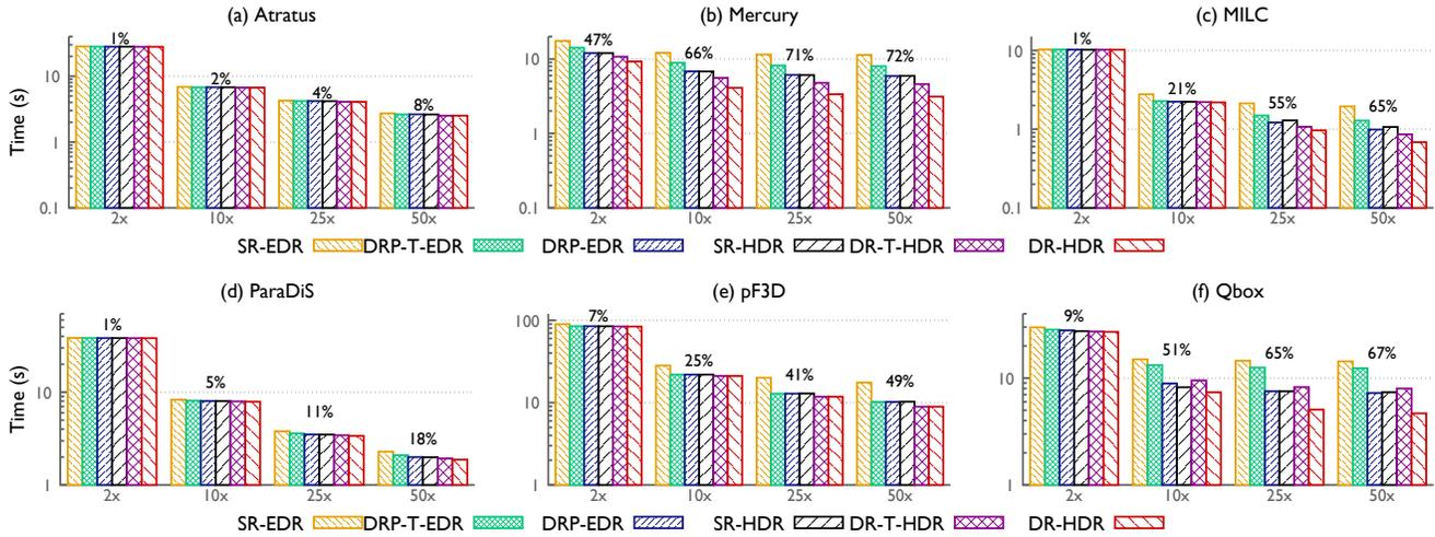
**Figure 7: Analyzing the effect of network configurations on scenarios with different computation scaling. % difference between the best and the worst configuration is shown.**
