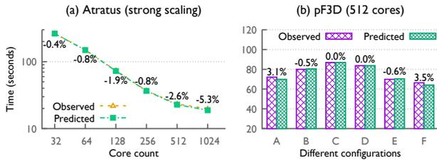
**Figure 5: Prediction accuracy is high for latency-bound Atratus and bandwidth-bound pF3D.**
