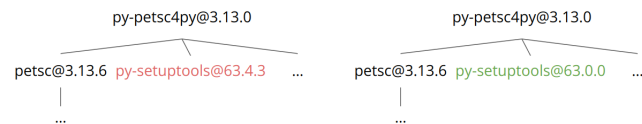
Figure 13: An example improvement using the new concretizer. Changing the setuptools version, which further propagates version changes to other Python packages, leads to a successful build (on the right).
