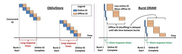
Figure 2: **Reducing response time.** Because Burst ORAM (right) does much less online IO than ObliviStore (left) and delays offline IO, it is able to respond to ORAM requests much faster. In this (overfly simplified) illustration, the bandwidth capacity is enough to transfer 4 blocks concurrently. Both ORAM systems do the same amount of IO.
