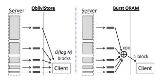
Figure 3: **Reducing online cost.** In ObliviStore (left) the online bandwidth cost is  $O(\log N)$  blocks of IO on average. In Burst ORAM (right), we reduce online IO to only one block, improving handling of bursty traffic.
