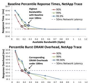
Figure 11: (Top) Insecure baseline (no ORAM) p-percentile response times for various p. (Bottom) Overhead (difference) between insecure baseline and Burst ORAM's p-percentile response times. Marked nodes show that when baseline p-percentile response times are < 100ms, Burst ORAM overhead is also < 100ms.
