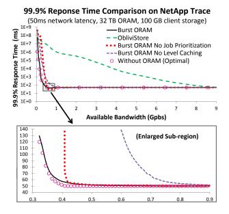
Figure 10: (Top) Burst ORAM achieves short response times in bandwidth-constrained settings. Since Oblivi-Store has high effective cost, it requires more available client-server bandwidth to achieve short response times. (Bottom) Burst ORAM response times are comparable to those of the insecure (without ORAM) scheme.
