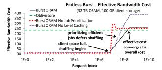
Figure 8: Effective bandwidth costs as burst grows. Burst ORAM handles most bursts with  $\sim 1X$  effective cost. Effective costs converge to overall costs for long bursts.
