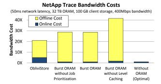
Figure 12: To achieve shorter response times, Burst ORAM incurs higher overall bandwidth cost than Oblivi-Store, most of which is consumed during idle periods. Level caching keeps bandwidth costs in check. Job prioritization does not affect overall cost, but does reduce effective costs and response times (Figures 8, 10).
