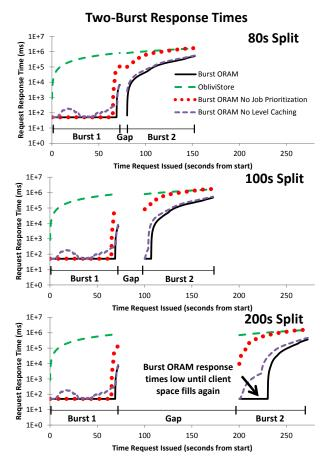
Figure 9: Response times during two same-size bursts of just over 2<sup>17</sup> requests spread evenly over 72 seconds. Client has space for at most 2<sup>18</sup> blocks. No level caching causes early spikes due to extra early shuffle reads.
