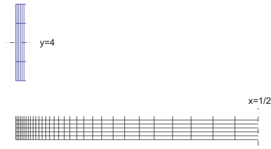
Fig. 3.1. Details of grid (to scale) showing the high aspect ratio rectangles in the two coordinate directions.
