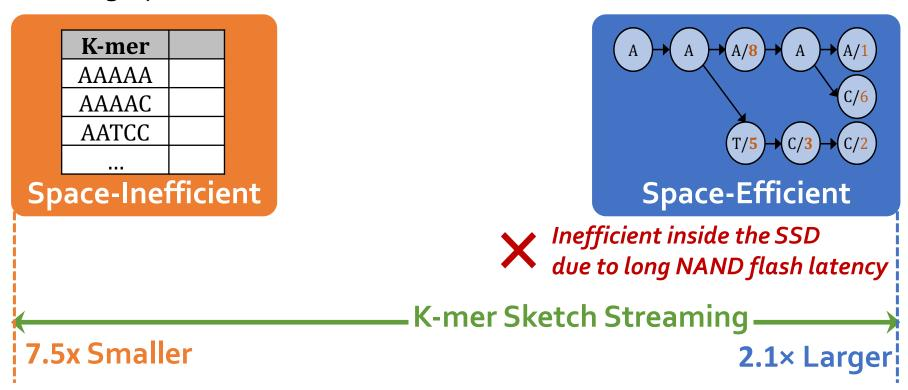
K-mer Sketch Streaming is much more suitable for in-storage processing due to its streaming accesses
