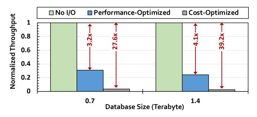
I/O data movement causes significant performance overhead
