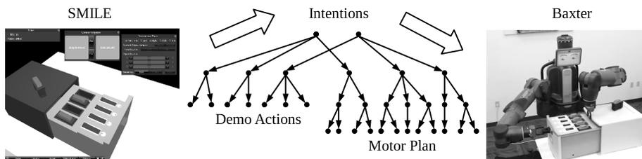
**Fig. 1.** Our IL framework. Demonstrations are recorded in SMILE (left) and imitated by a robot (right). Hierarchical intentions (center, explained below) are inferred bottom-up using causal reasoning (left block arrow). During imitation, intentions are decomposed top-down into new actions and ultimately motor plans (right block arrow).
